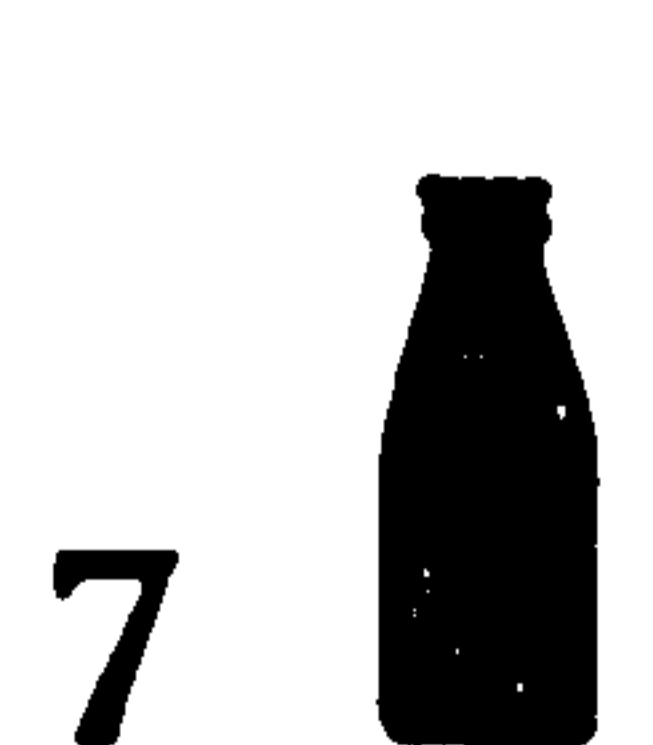
7 Released from the blow mould, the bottle travels to the lehr.
