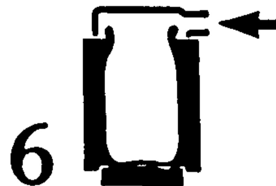
6 Compressed air is forced into the parison, forming the jar.
