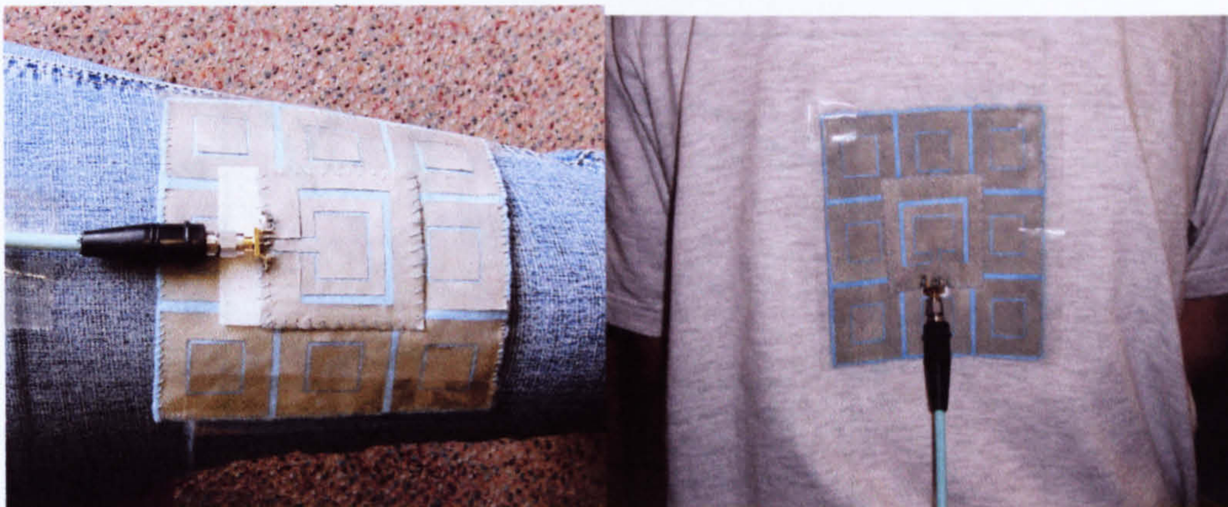
Figure 6.6 Dual-band EBG antenna mounting on the thigh and back
