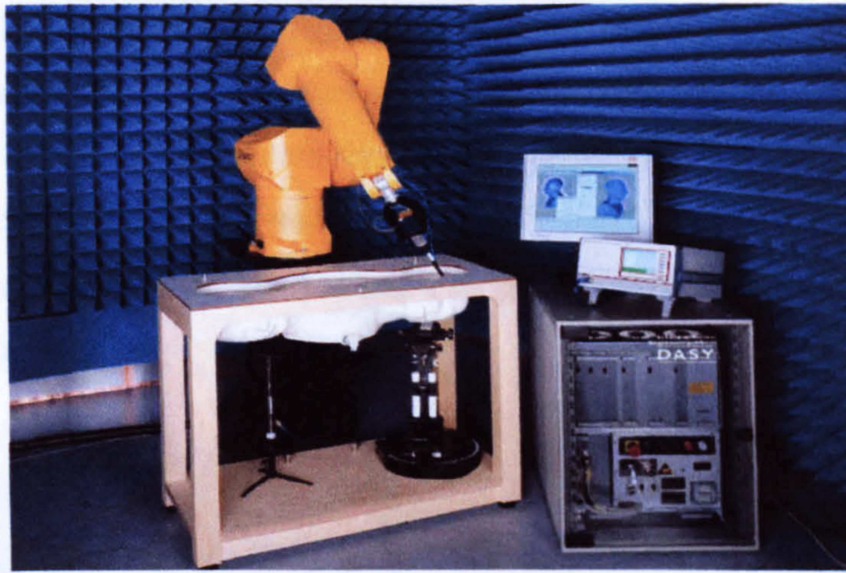
Fig 6.17 DASY4 system structure [13]
