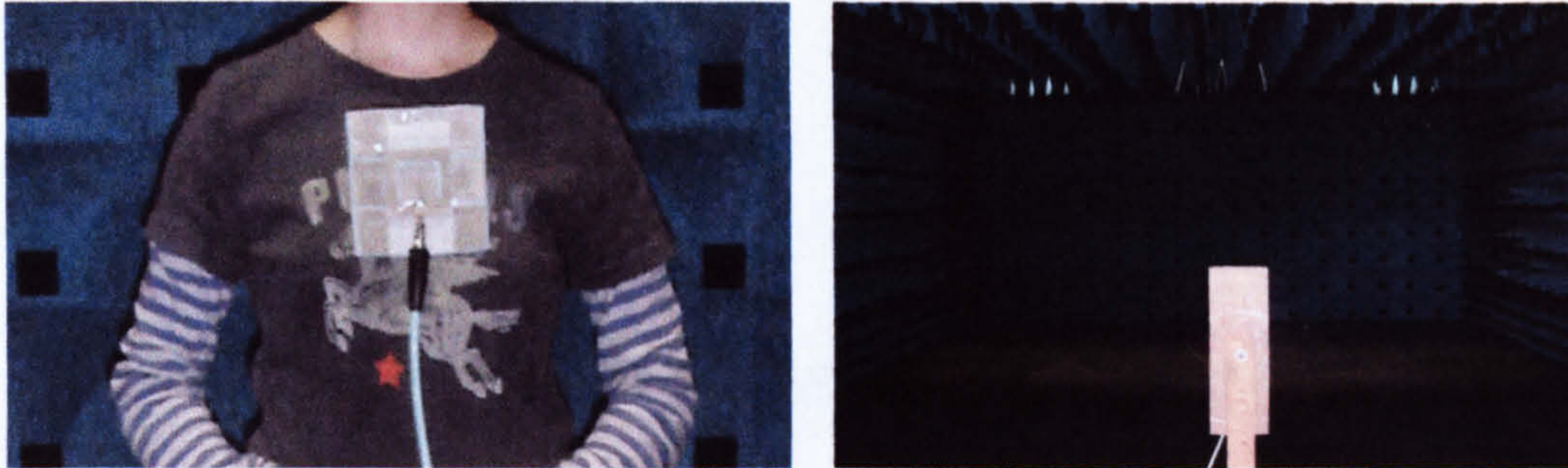
Figure 6.9 Measurement set up for antenna on body in anechoic chamber
