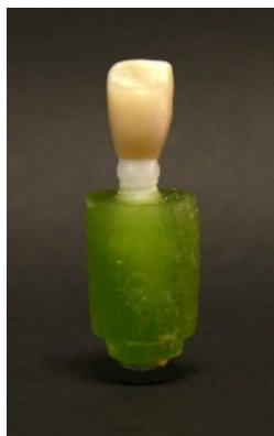
Figure 64. . Implant-abutment-crown assembly embedded in resin block
