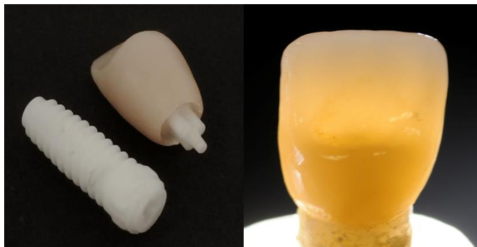
Figure 68. Outcome of dynamic fatigue test.
