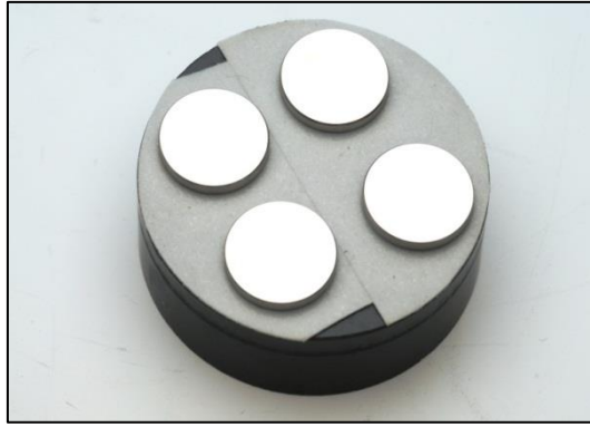
Figure 77. Mirror polished grade II cpTi discs.
