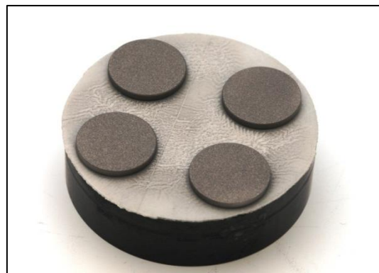
Figure 79. Sandblasted cpTi discs with Alumina abrasive particles (250-500µm).
