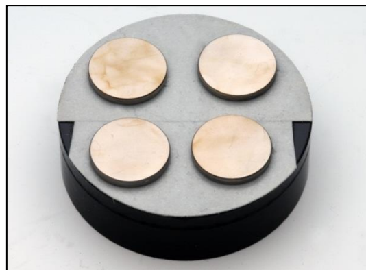
Figure 78. Grade II cpTi discs after two acid pickling cycles .
