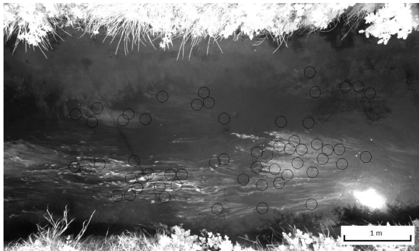
Figure 11. NIR reflection at water surface (light haze in top half of the reach); Band NIR(R72), site 2.
