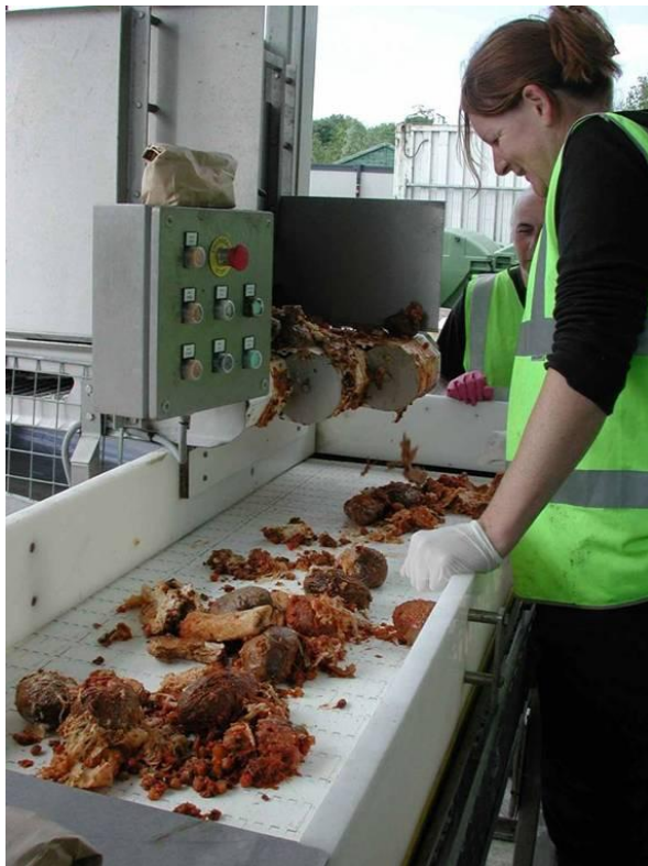
Figure 6: Clare and John from the Waste Neutral Operations Team carrying out final inspection of food waste before shredding and composting.
