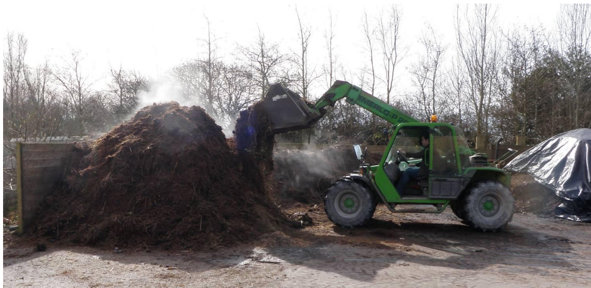
Figure 16: Eden food waste compost is used as an activator feedstock in our green waste composting operation. Here a recently mixed heap is being turned and aerated.
