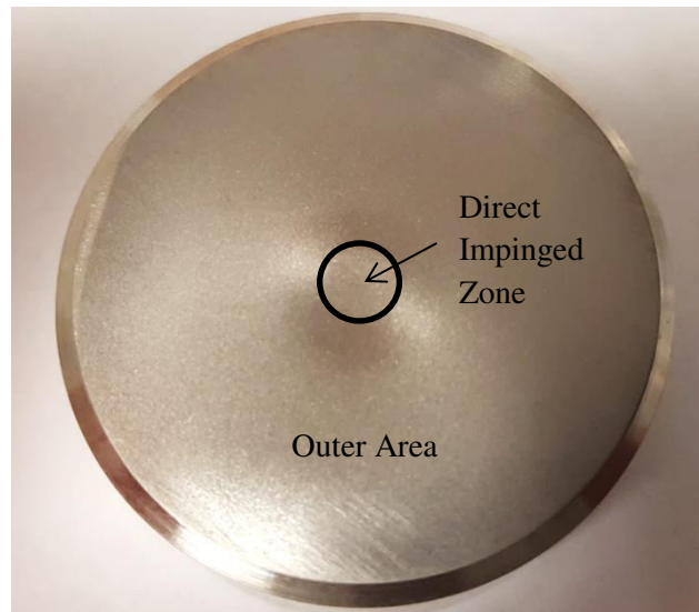
Figure 7: Wear scar on SS316 after 1 hr test at 90° impingement, highlighting the two distinct wear zones
