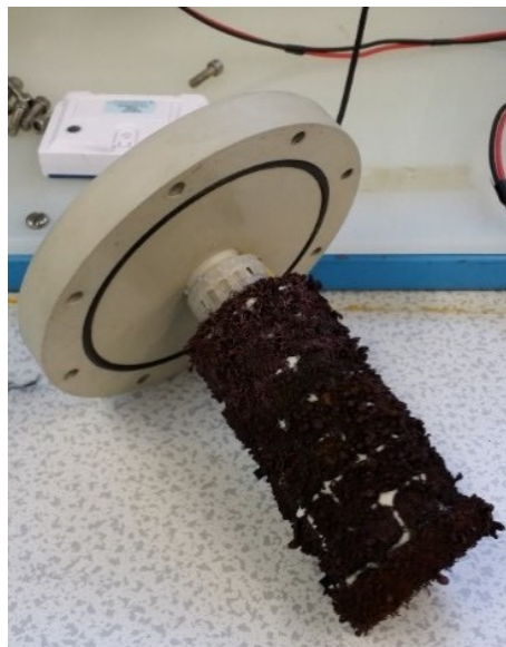
Figure 3: Images of the carbon felt cathode before and after electrowinning.
