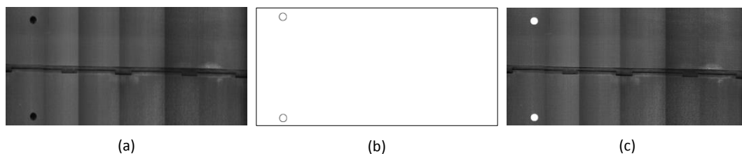
Figure 3 Trepanned hole detection using Hough Transform for circle detection – (a) original image (b) Binary result of circle detection algorithm (c) circles detected overlaid on original and filled in
