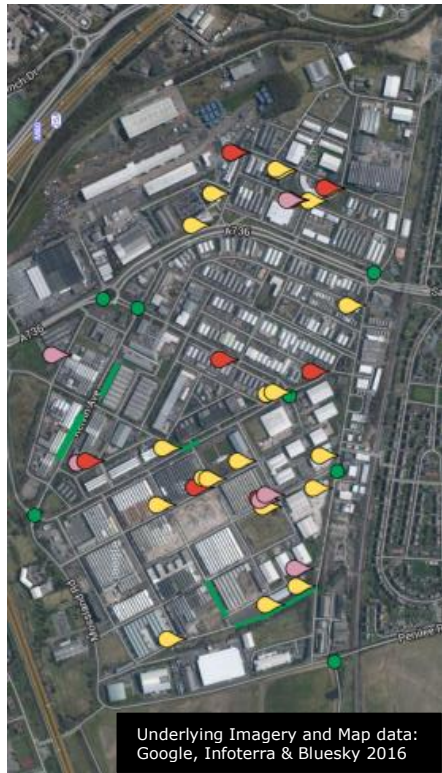
Figure 2. Manual log (red=sudden stops / green = potential false positive zones (bumps, roundabouts, etc.)) plus warnings from phones (yellow=S3Mini / pink=Nexus5)
