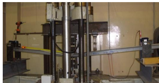
(c) Test photograph of uplift loading direction for U-61-N3 specimen
