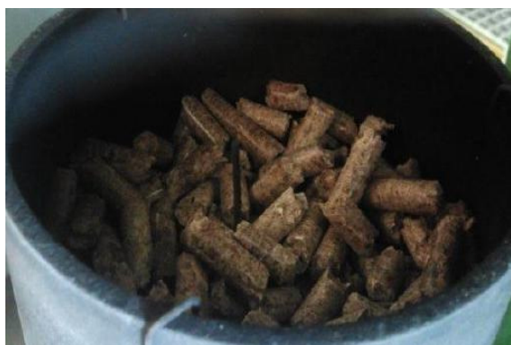
54 55 56 57 58 59 60 61 62 63 64 65 Fig. 1. Sample holder with Biomass inserted in the reactor (left); Labr eactor setup (right)
