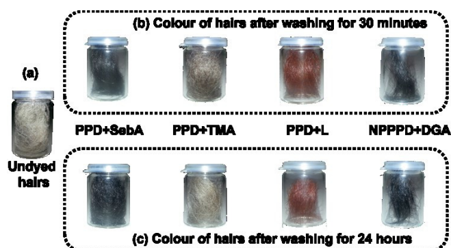
Figure 3. (a) Undyed hairs. (b and c) Dyed hairs after washing for 30 minutes and 24 hours respectively.
