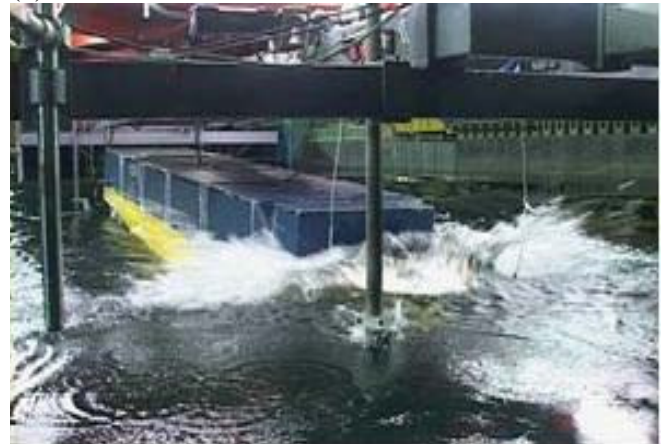
Figure 3. Key information for WILS II 10,000 TEU Container Ship (a) general particulars (b) body plan (c) mass distribution of segmented model (d) configuration of model ship setup and locations of sensors – 1/60 scale (e) hydrodynamic testing (NB : k_{xx} , k_{yy} and k_{zz} represent the radii of gyration of roll, pitch and yaw).
