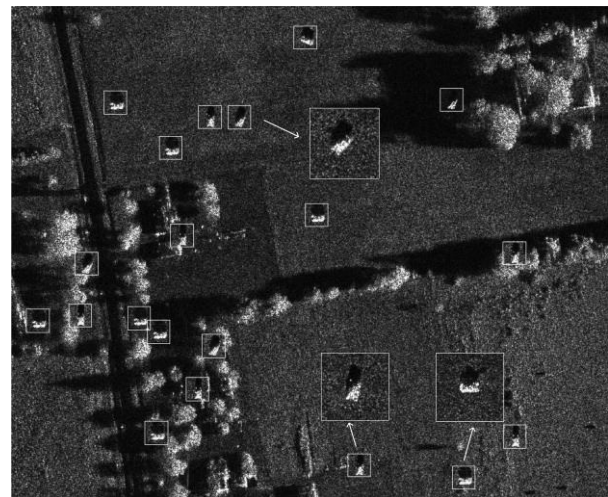
Fig. 9 shows a composed SAR image when SCR = 2.0 In order to observe their locations easily, the targets are marked
