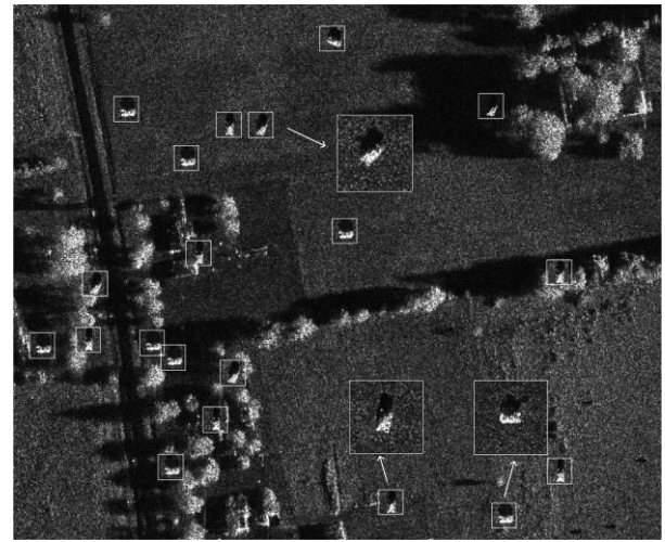
Fig. 9 Composed SAR image with SCR=2, which includes 20 real targets labeled by red rectangle
