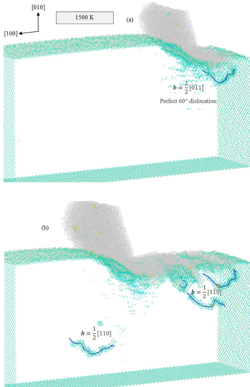
Fig. 3. Dislocation nucleation while cutting the (010) plane at 1500 K at a cutting distance of (a) 10 nm and (b) 20 nm.
