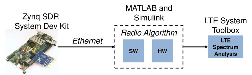
Use Simulink to partition algorithm into HW and SW
