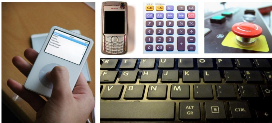
Figure 6: Buttons used in consumer products (Clockwise from top left – Apple iPod, Nokia push-button mobile telephone, standard calculator interface, emergency stop button, Toshiba laptop keyboard)
