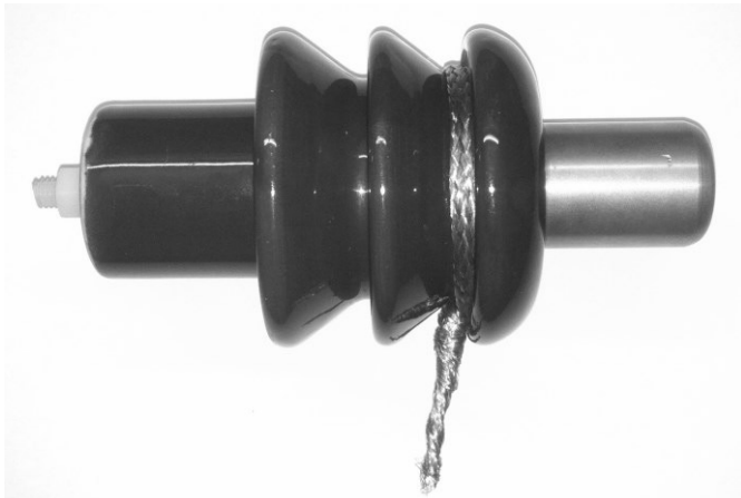
Fig. 2. Surface discharge sample. A ceramic transformer bushing with the high voltage terminal connected via the brass fitting and a ground wrapped part way down the bushing.
