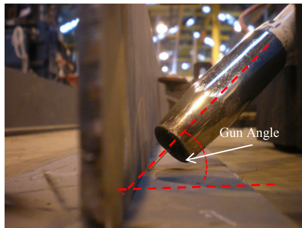
Figure 3: Diagram showing gun angle orientation
