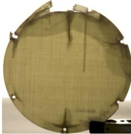
Fig. 18. Damaged test plate after the shock loading in CST [4].
