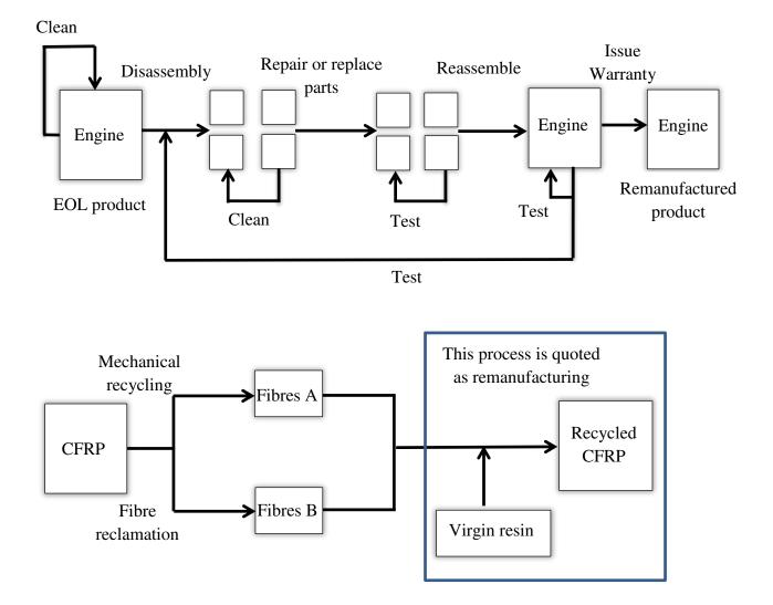
Figure 2 – Standard remanufacturing process carried out on an engine and the general remanufacturing process in relation to CFRP as described within literature. Noting that mechanical recycling will produce chopped and powered fibres with traces elements of resin, hence fibre a and fibre b denomination.
