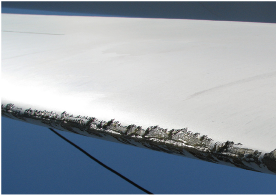
Figure 1: An example of leading edge erosion [2]
