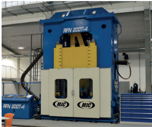
Figure 4. Rotary forging system capable of making parts up to 400 mm diameter.
