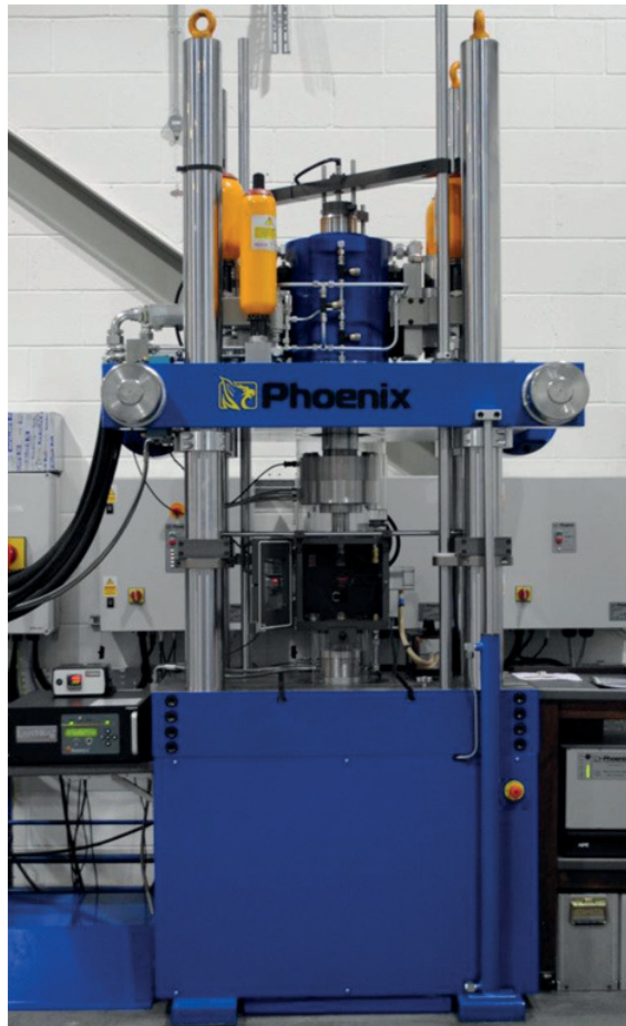
Figure 2. High rate compression testing machine used for obtain baseline data for forging models.
