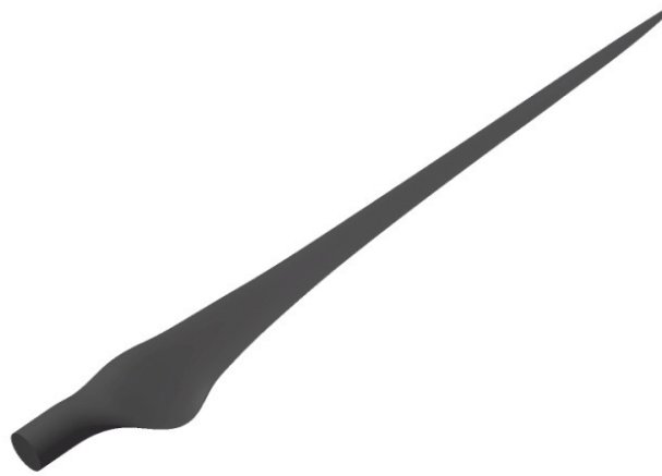
Figure 3: Isometric view of the optimized 60 kW blade
