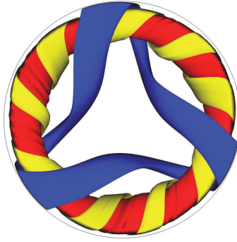
Figure 7: Dominating KAM tori (not all tori are shown) for \text{Re} = 2600 : T_3^3 (blue), the core T_{\text{core}} (red) and T_{1\alpha}^9 (yellow). The circle indicates the free surface.
