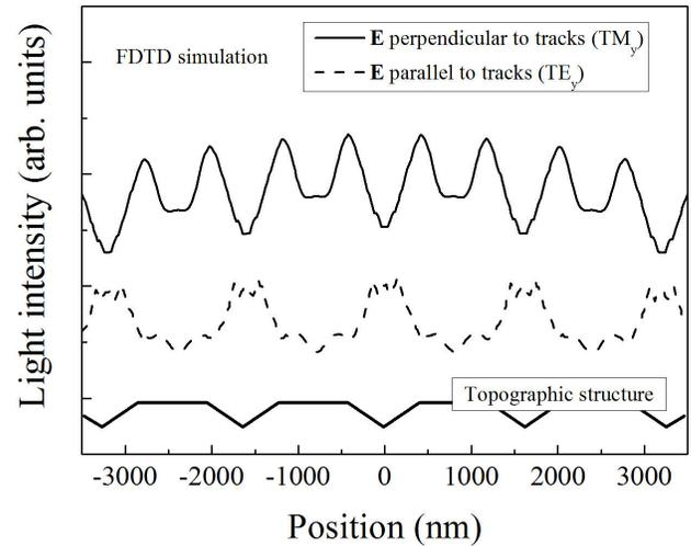
FIGURE 4. FDTD simulations of the SNOM light intensity profiles. Continuous line: electric field polarization parallel to the tracks direction. Dashed line: electric field polarization perpendicular to the tracks direction. At the bottom, the simulated topographic profile is drawn.
