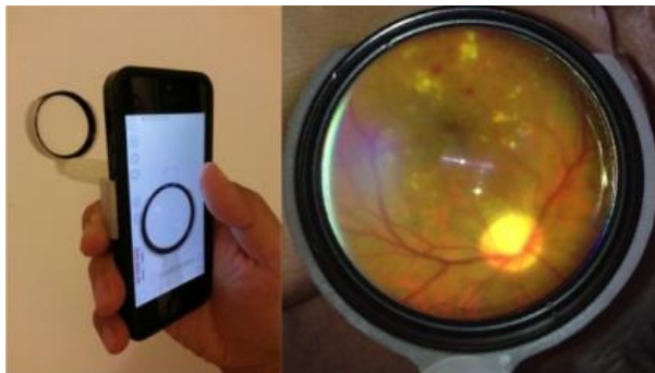
Figure 3 –The 3d printed smartphone retinal adapter for monocular indirect ophthalmoscopy developed by Myung et al. [35] on an iPhone 5 (Apple Inc.) (left). Diabetic macular edema can be photographed using this lens-to-phone mount (right). Reproduce with permission from [35].
