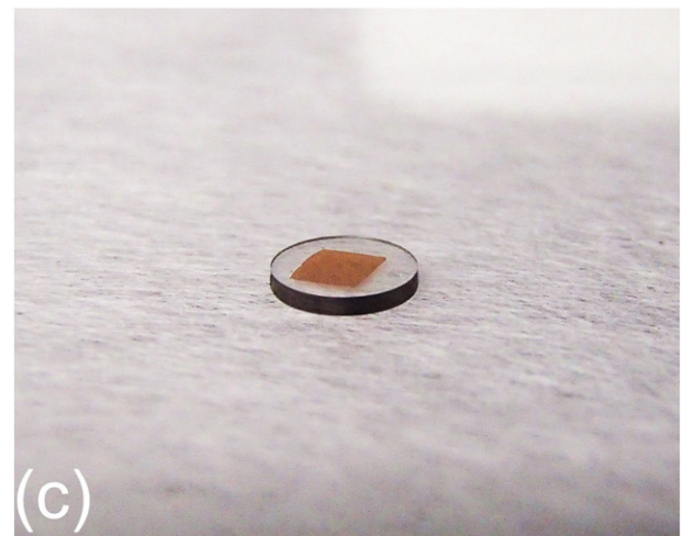
Fig. 4. Processed samples: (a) Sample following polishing and etching of the InP substrate to the InGaAs layer; (b) InGaAs buffer layer etched to reveal the II–VI etch stop. (c) A sample capillary bonded to a 4 mm diameter diamond.
