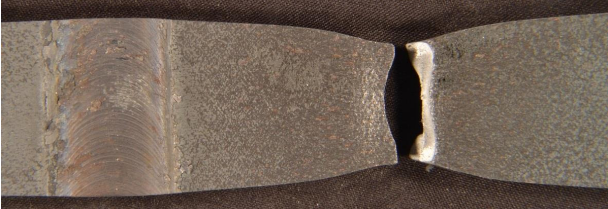
Fig. 7 Tensile sample fracture in parent material
