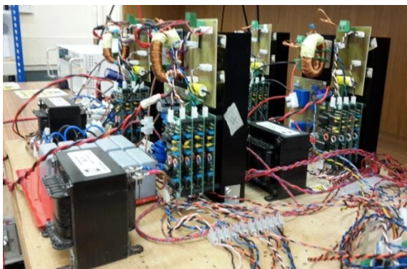
Fig. 10. ISIPOS connected full-bridge DC/DC converter test rig
