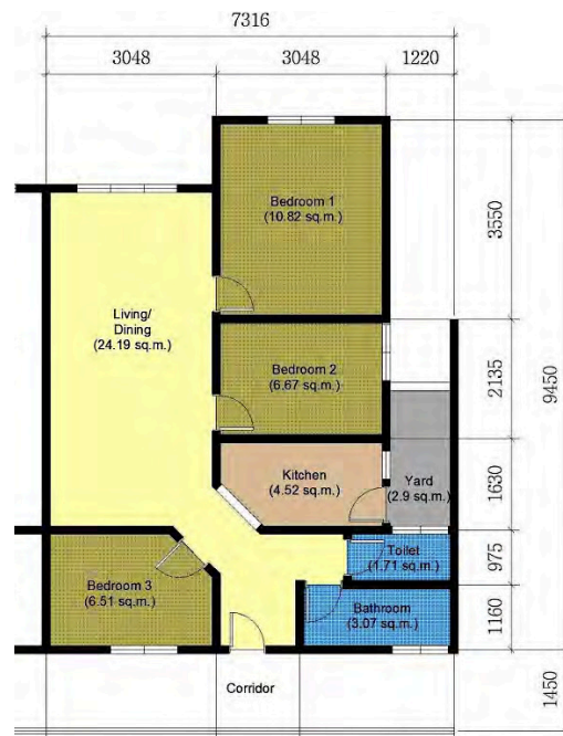
Figure 4. Layout plan of a PHP 2000 (Source: Redraw by the author from Goh & Ahmad, 2011)
