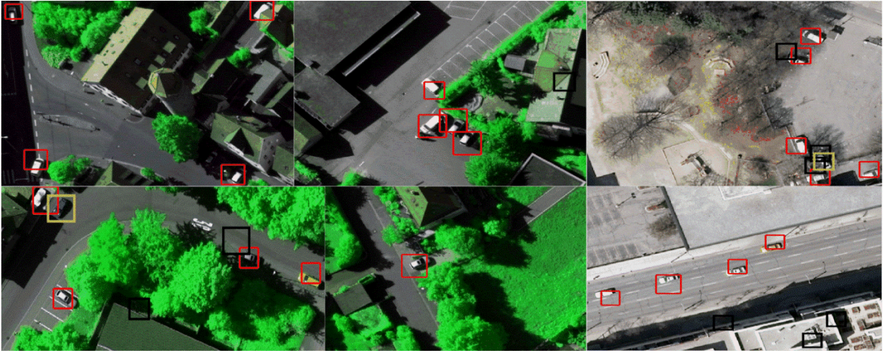
Fig. 14. Examples of vehicle detection in the ISPRS dataset.
