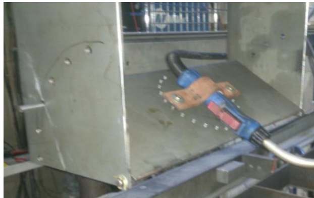
Figure 4 : Jig for setting Travel and Gun Angle
