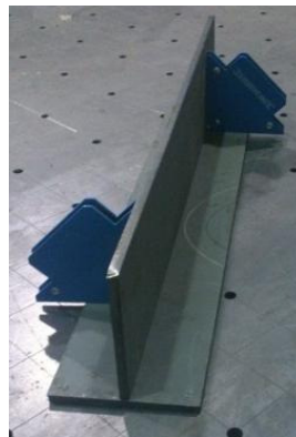
Figure 5: Example of DH36 Mild Steel 'T' test piece
