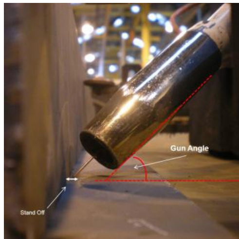
Figure 6 : Image showing gun angle and stand-off measurement
