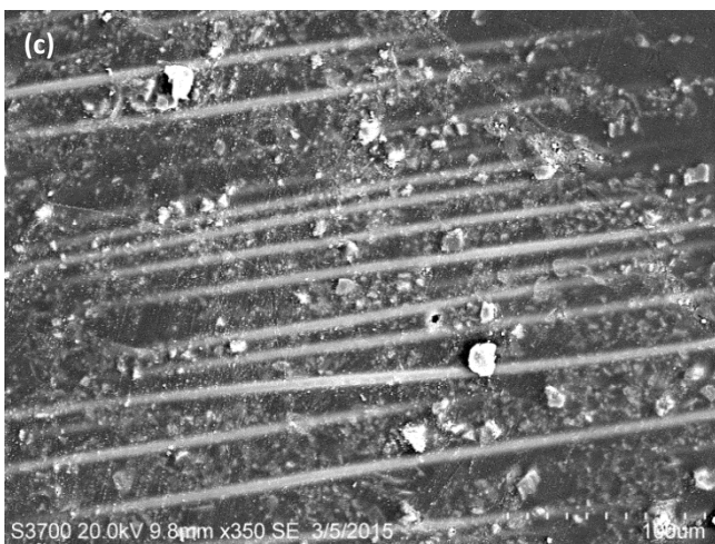
Figure 6 – sample after a test in salt only solution at 60° impact angle (a) site 1, (b) site 2 and (c) site 3
