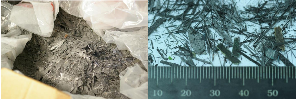
Figure 4 Left: Shredded carbon/epoxy prepreg laminate (secondary size reduction), Right: Composite ready for feeding to the fluidised bed
