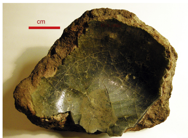
Fig. 10. Crucible fragment from Lisht with thick layer of glass.
