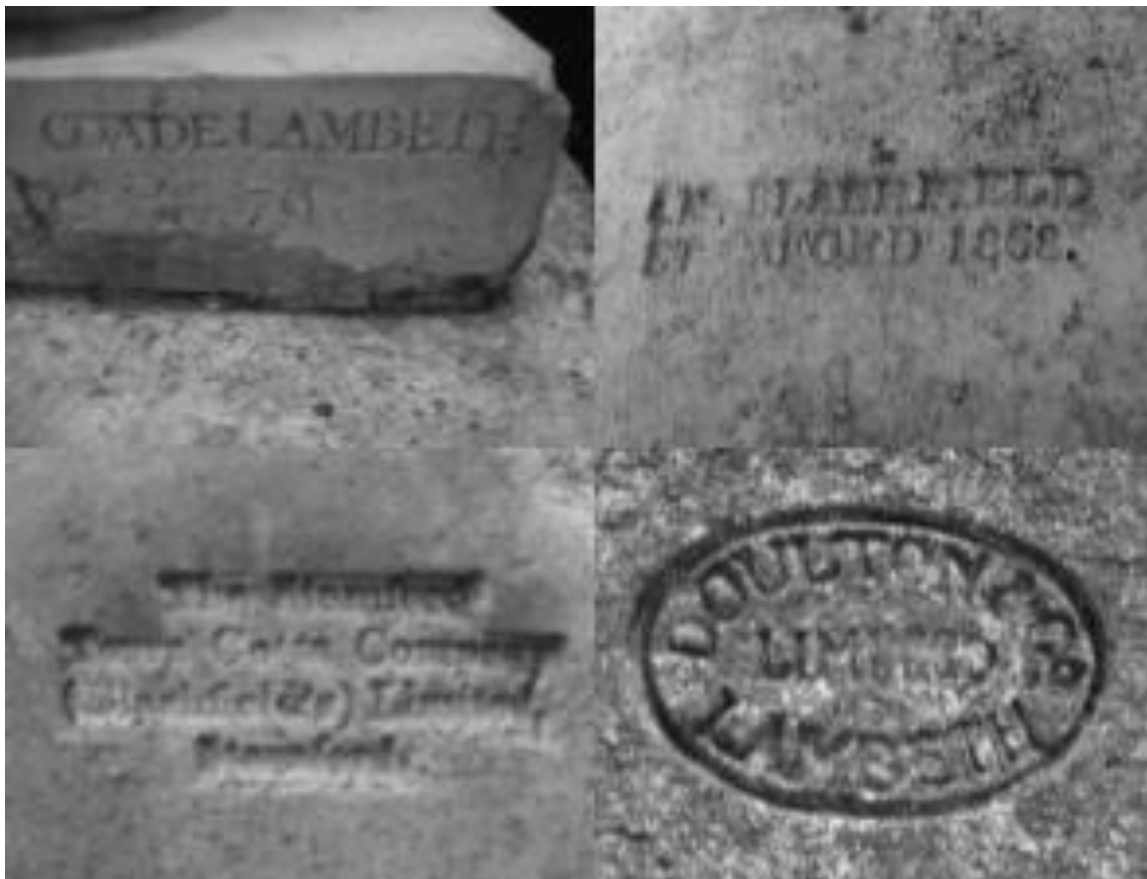
Figure 1 Examples of manufacturer's stamps on ceramic objects. Clockwise from the top left: Coade Lambeth 1779 (ACA, ACB, ACC); J.M. Blashfield Stamford 1868 (CABA, CABB, CAB); The Stamford Terra Cotta Company (Blashfield) Limited, Stamford (1872-5) (BA, BC); Doulton & Co Ltd Lambeth (1890-1902)(CADA, CADB, CAD, CADD)
