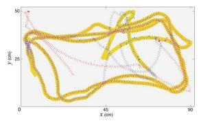
Figure 6. Trajectory of three robots. Leader (yellow shadow) and two follower robots (dashed lines with red and blue colors).
