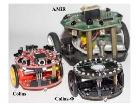
Figure 1. Colias-Φ, Colias and AMiR mobile robots developed for swarm robotic applications
