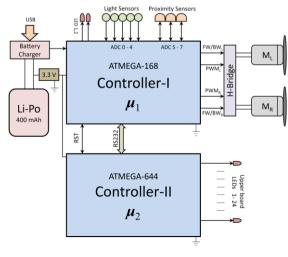
Figure 3. Architecture of Colias- $\Phi$
