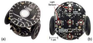
Figure 2. Colias-Φ micro robot platform developed for pheromone communication system
