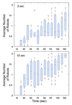
Figure 7. Average number of robots on the pheromone trail in different evaporation delays ( $e_{\phi}$ = 5 and 10 sec) with 3 robots (one leader and 2 followers).
