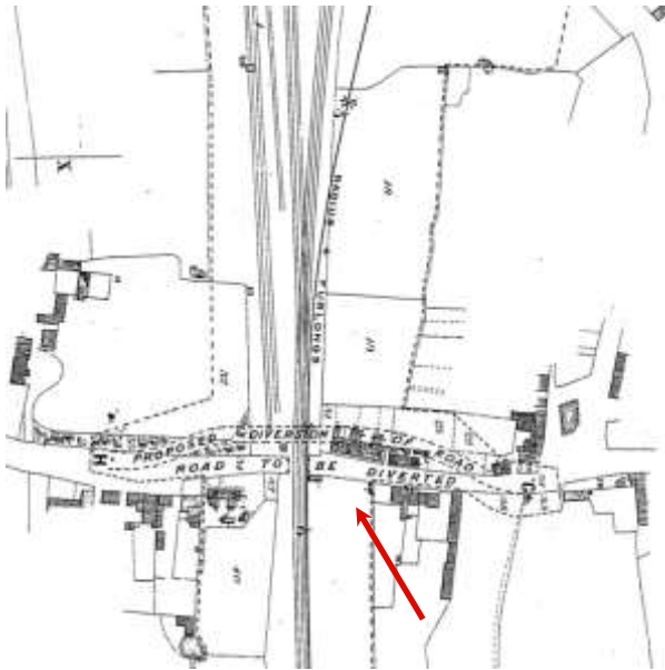
Figure 50: Pre 1884 plan for construction of bridge over the railway after accident over level crossing. Arrow marks test pit position
