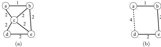
Figure 5: Contraction hierarchies preprocess the original graph (a) by removing certain nodes and introducing pre-computed shortcuts (dashed line). The final graph (b) is more sparse and therefore easier to search. (Adapted from (Sturtevant and Geisberger, 2010).)
