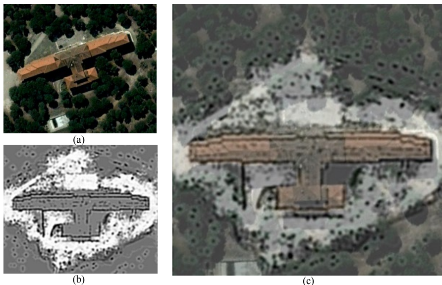
Figure 27 – (a) Aerial view of the scanning site. (b) resulting 2D navigation map. (c) Comparative image between the obtained 2D Navigation map and the aerial view of the environment
