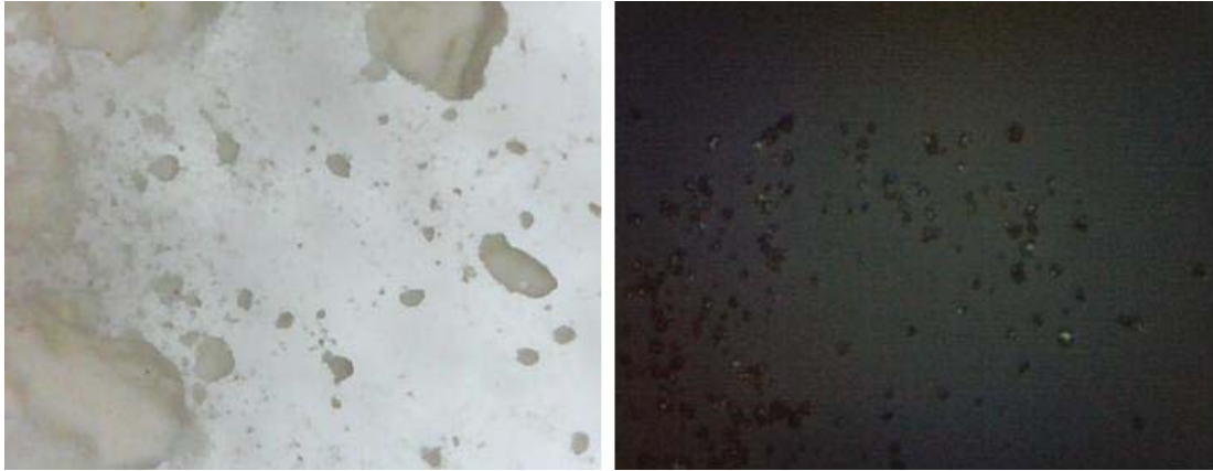
Figure 2. F. White pigment at x220 magnification using light microscopy (left); F. White pigment at x400 magnification under polarised light (right) showing birefringence.
