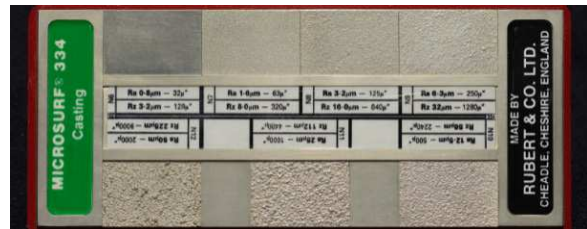
FIGURE 5. Rubert Microsurf 334 comparator test panel.
