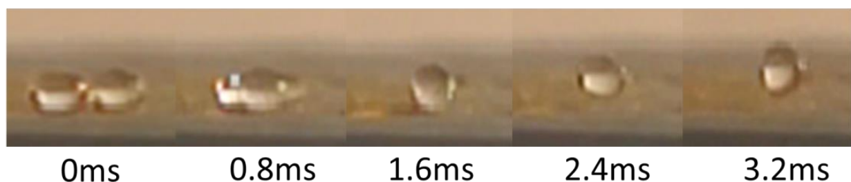
Figure 6: Experimental validation of jumping phenomenon on superhydrophobic surface, droplet with initial radius 515\ \mu\text{m} jumping upon coalescence, droplet velocity \bar{v}_j = 0.039\ \text{m/s} .
