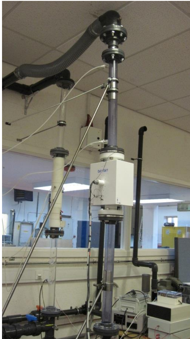
The IFT flow meter in the flow loop
