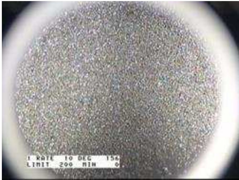
Fig. 22. A hot stage image of indium powder after fusion at 156°C (sample mass, 2mg; heating rate, 10°C min -1 ; atmosphere, nitrogen)
