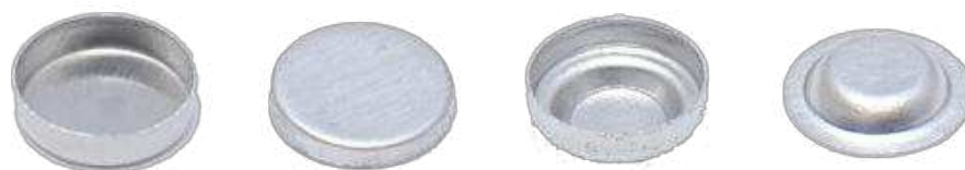
Fig. 19. TA Instruments non-hermetic (left) and hermetic (right) Al pans. 33
