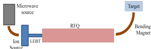
Figure 1: Schematic overview of our proposed accelerator isotope system.
