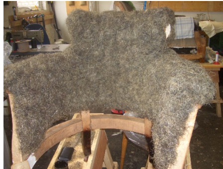
Figure 2: The stripped chair frame with new webbing (left-hand image) and (right-hand image) the chair frame with the beginnings of the horse hair stuffing applied to the inner back and sides (traditional materials and techniques).
