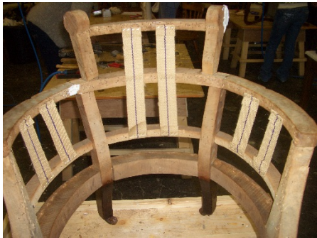
Figure 2: The stripped chair frame with new webbing (left-hand image) and (right-hand image) the chair frame with the beginnings of the horse hair stuffing applied to the inner back and sides (traditional materials and techniques).
