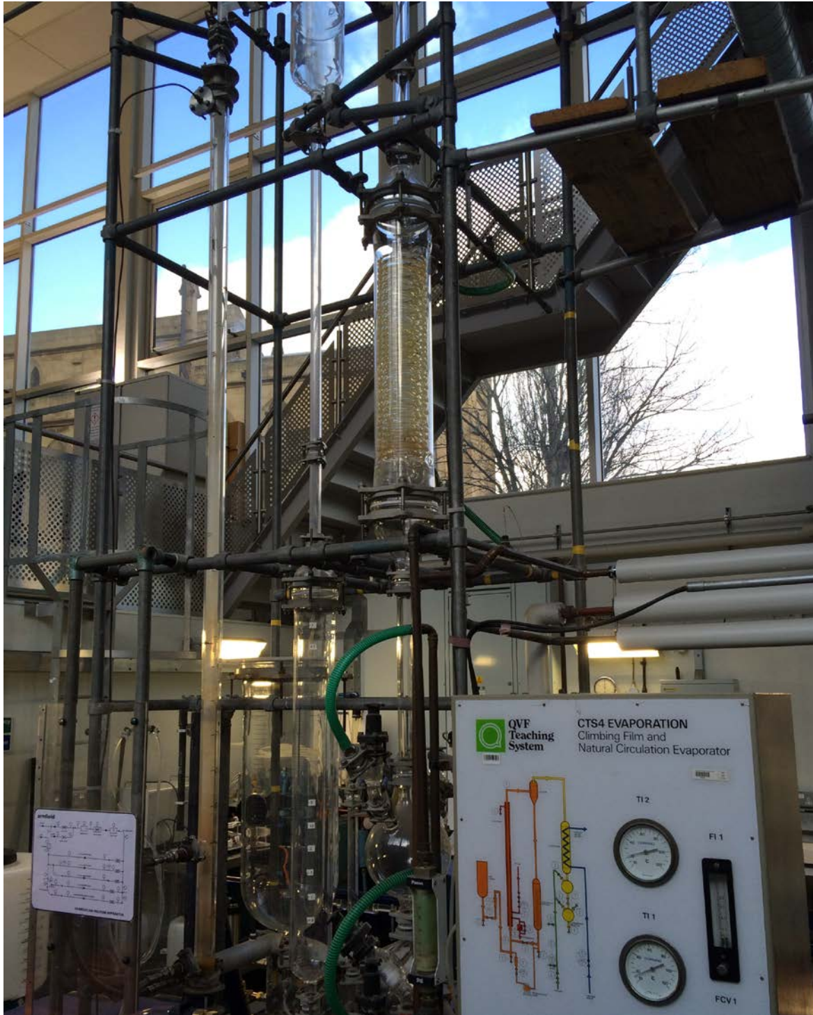
Figure 4: Climbing film evaporator in the pit area of the chemical engineering lab.
