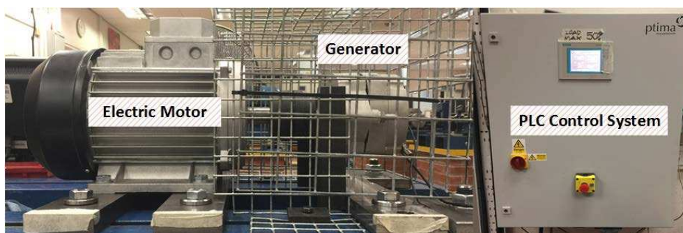
Figure 7. View of experimental generator test set up.
